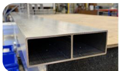
Final rear-frame profile design/Longitudinal section
